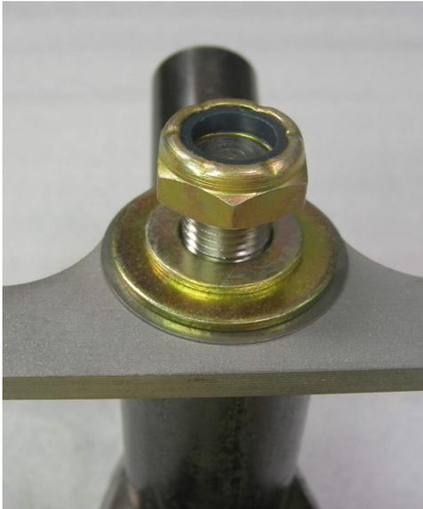
The center photo shows the placement of the optional shim. The shim is **OPTIONAL**. It is simply used to fill small gaps caused by wear or part variation between different manufacturers. As the bushing in the mounting socket wears down in height, you may add a shim washer if you like. Unless bushing wear is severe, the shim washers are for aesthetics only and do not affect normal operation.
